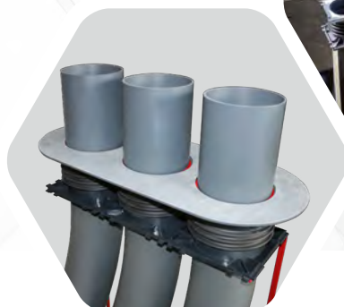
KRASO® Cable Inlet Box System KDS 150 available with KRASO® Trowel Flange roughened plastic-trowel flange for the integration into the floor sealing / sealing sheets
