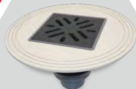
KRASO® Yard/Parking Level Drain Type 1.5 with trowel flange with dovetail groove (only for welding sheets, not for resin coating)
